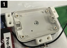
1 Take front cover and place on fixture as shown. Ensure LED HOLE is bottom half!
