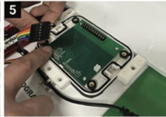
5 Insert rubber seal. FLAT SURFACE UP! Ensure no fouling.
