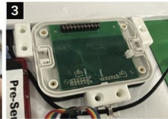
3 Place PCB in orientation shown (ANTENNA TOP HALF) ensuring holes are aligned
